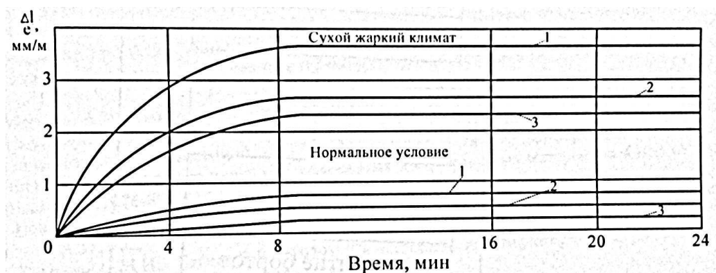
Picture 4 - Kinetics change the initial plastic shrinkage ( W/C = 0,50 , the consumption of cement, 370 \text{ kg/m}^3 ). 1 1 and 1 without additives; 2 1 and 2, with the addition of 0,40%; 3 1 and 3, with the addition of 0,60%.
